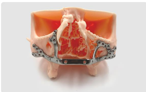
Fig. 1: A 3D-printed anatomical model of a maxilla showcasing a custom-designed metal implant for maxilla reconstruction. The implant, precisely fitted to the anatomical structure, demonstrates the advanced design capabilities facilitated by Simq's simulation software.
